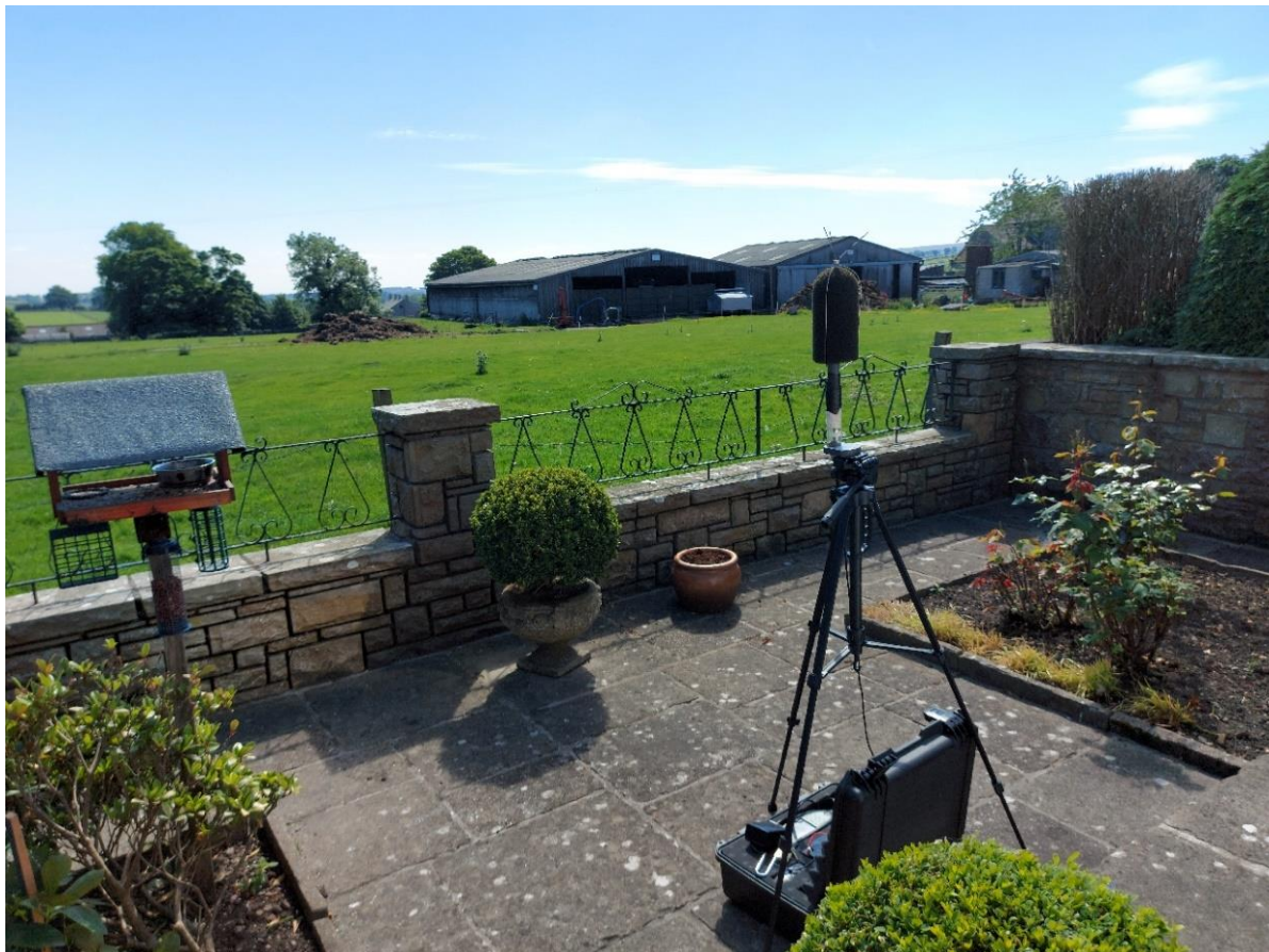
Plate 23: Noise monitoring equipment at Kilmond View
