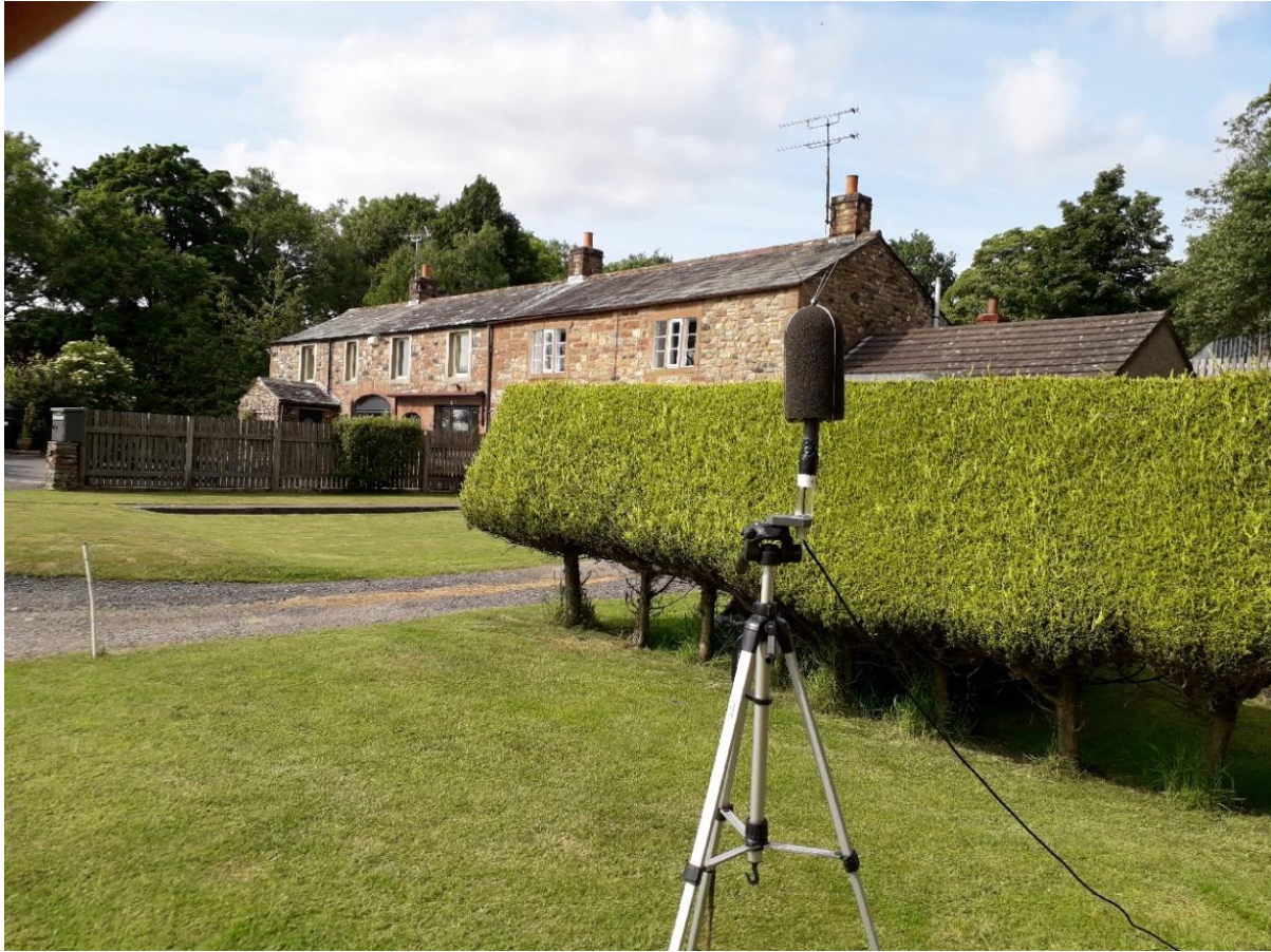
Plate 19: Noise monitoring equipment at Walkmill
