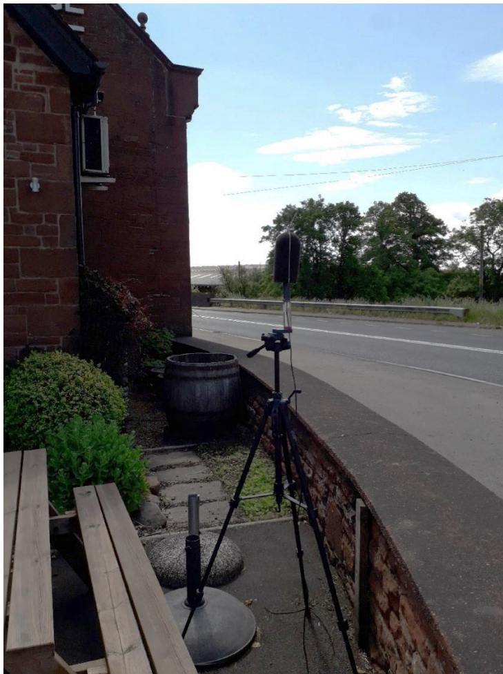
Plate 17: Noise monitoring equipment at Bridge Hotel
