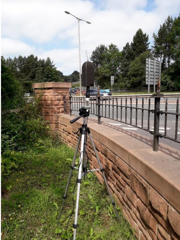
Plate 3: Noise monitoring equipment at Skirsgill Lodge
